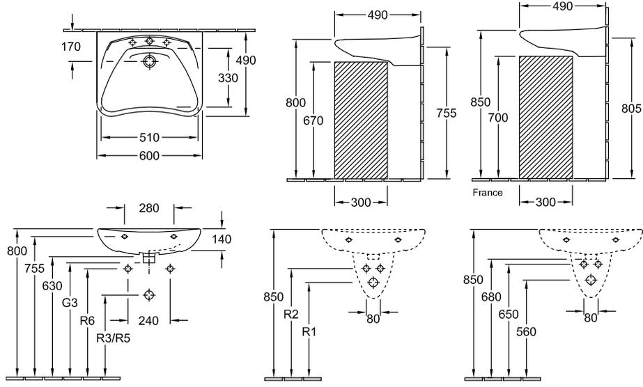
R3 Installation in acc. with DIN 18040 with standard space saving siphon
